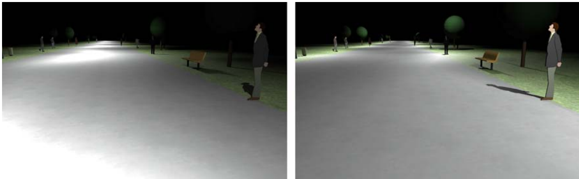
Figure 1. Current road lighting method in practice (left) and proposed concept (right). Headlights are excluded.
